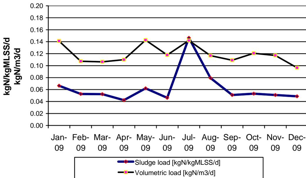
Figure 2.18. Nitrogen load to aeration, 2009.
