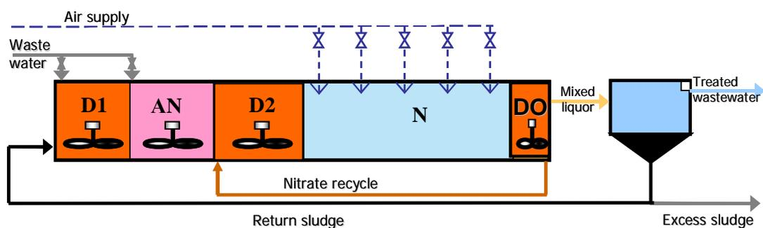
Figure 3.4. Johannesburg process (JHB) for biological nitrogen and phosphorus removal.
