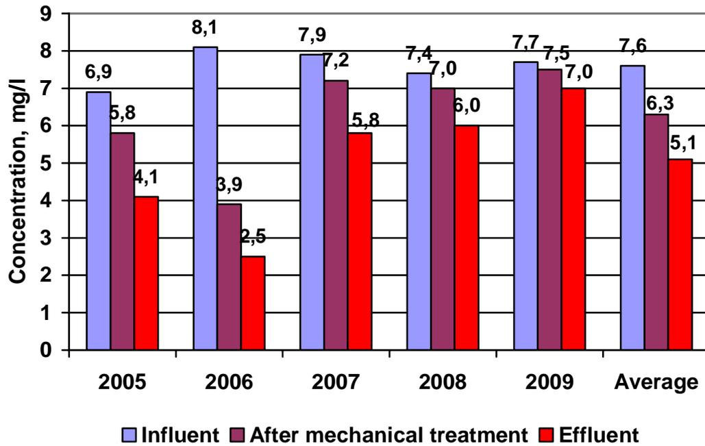
Fig.2.5. Phosphate phosphorus (PO<sub>4</sub>-P) concentrations 2005-2009
