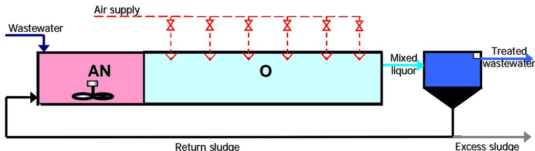
**Figure 3.5. AO (anaerobic-oxic) process for biological phosphorus removal.**
