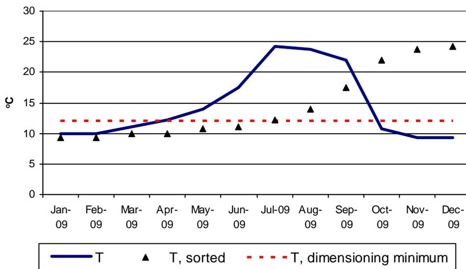
Figure 2.8. Influent wastewater temperatures, 2009.
