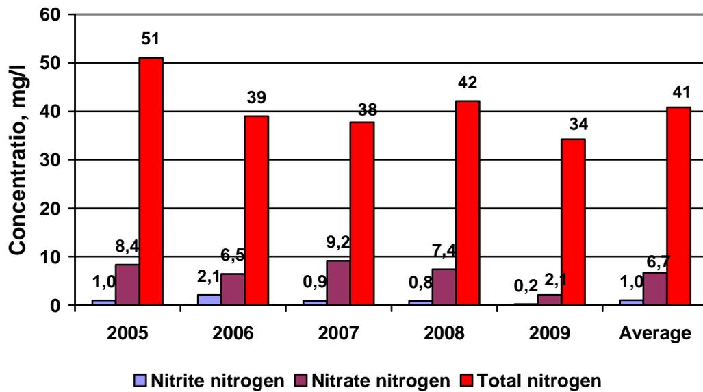
Fig.2.4. Concentrations of nitrite nitrogen, nitrate nitrogen and total nitrogen after secondary clarifiers 2005-2009
