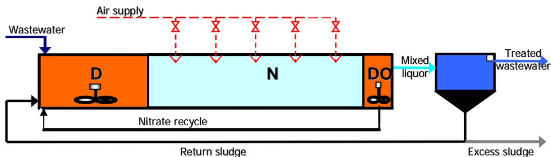
Figure 3.3. Denitrification-nitrification (DN) process for biological nitrogen removal.
