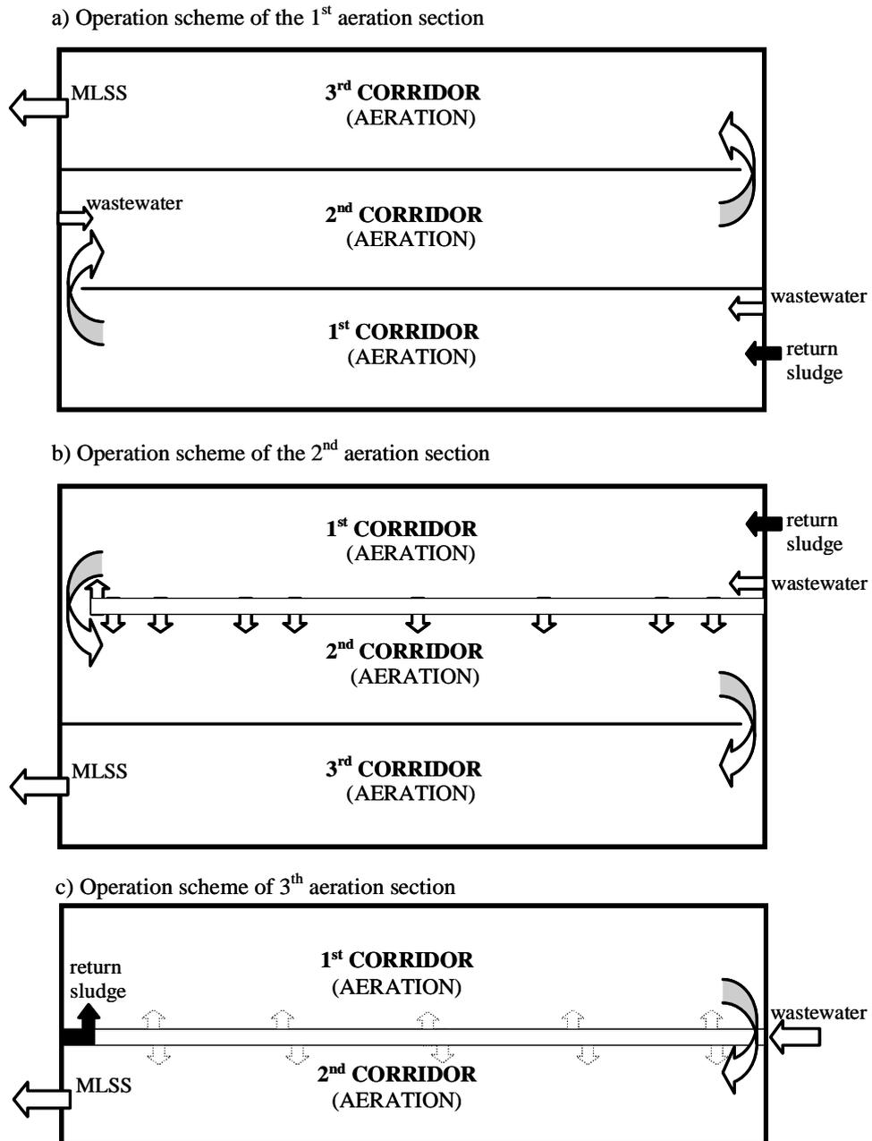
**Figure 2.12. Operation schemes of aeration tanks at Brest WWTP**
