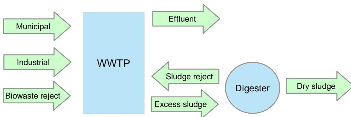
**Figure 3.1. Simplified phosphorus balance of the WWTP and digestion plant**
